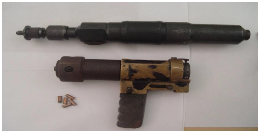
Captive bolt pistol and bullets
